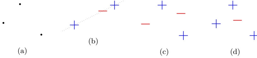
Figure 3.3: (a) A set of 3 points shattered by linear threshold functions. (b) A dichotomy on a set of 3 points that cannot be realised by linear threshold functions. (c) & (d) No set of 4 points can be shattered by linear threshold functions.
